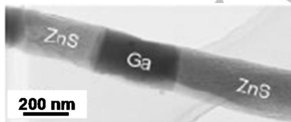
Figure 7. TEM image of a Ga/ZnS segmented NW within a silica shell. Reproduced with permission from Ref. [137].
